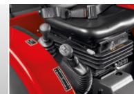
Integral, with 12 gears and assisted changes (8 FW + 4 RV) offers a choice of speeds in a logical sequence suitable for all uses, situations and terrain. Dry single-disk clutch.
