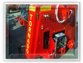
Application to the tractor through the Three Linkage
