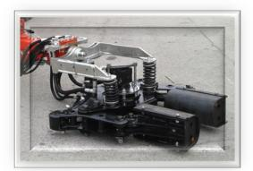
VIBRATING HEAD mod. P100 CLOSURE SYSTEM WITH TWO PARALLEL MOVABLE ARMS
